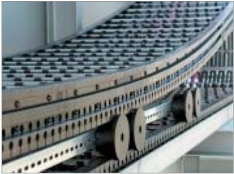
■ Flanged rolling castors – similar to railroad wheels – allow KabelSkate to be self-guiding.
